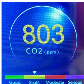
At 800 ppm for this particular monitor, the colour changes to **yellow** and this gives a warning. At about this point the ventilation is diluting exhaled breath by about a factor of 100.
