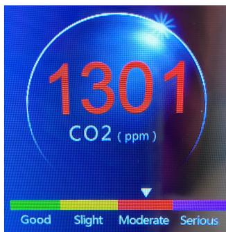
Above 1200 ppm the display changes to **red** and the CO<sub>2</sub> hazard is described as **Moderate**.
