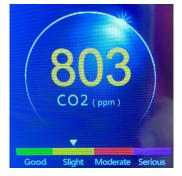
At 800 ppm for this particular monitor, the colour changes to yellow and this gives a warning. At about this point the ventilation is diluting exhaled breath by about a factor of 100.
